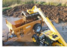
Constructed using **6mm** floor panel and **4mm** side panel for strength and durability. The standard **1.5m** wide body with a flared top creates a wider area for easy loading and less spillage.
