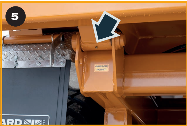
Grease Body Tipping pivots (2 Positions).
