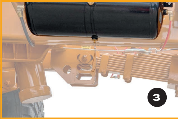
Drain water from Air reservoir.
