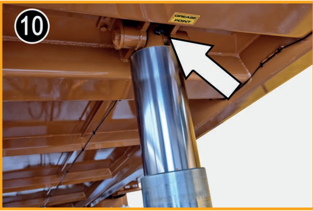
Grease Upper Tipping Cylinder Pivot.
