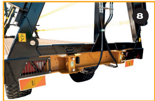
Check bolts securing head board / Ladders and other attachments for (2 positions).
