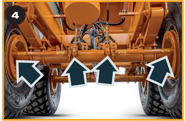
Grease Brake linkage pivots (4 Positions each Axle).
