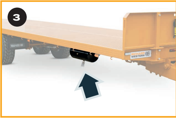
Drain water from Air reservoir.
